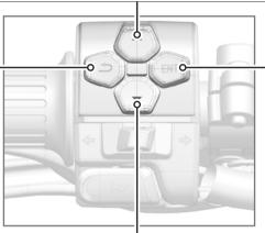
For Main interface: press it to enter the first-level menu, long press it to play the song. (When the bluetooth is connected).
