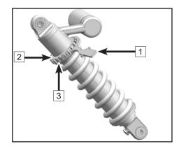
Rear shock absorber: K2C Rear shock absorber volume: 220 ± 2mL
