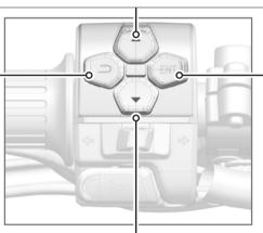
For Main interface: press it to enter the first-level menu, long press it to play the song. (When the bluetooth is connected).
